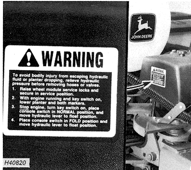
Hydraulic Manifold Cover
