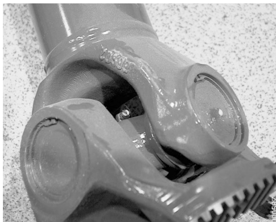
Grease nipple for universal joint, example
