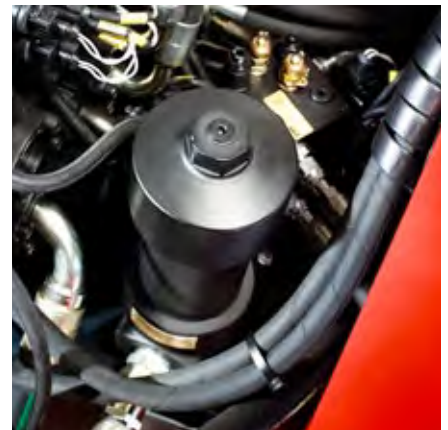
Improved placement of hydraulic filters.
