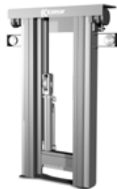
Triplex full free lift, free visibility
