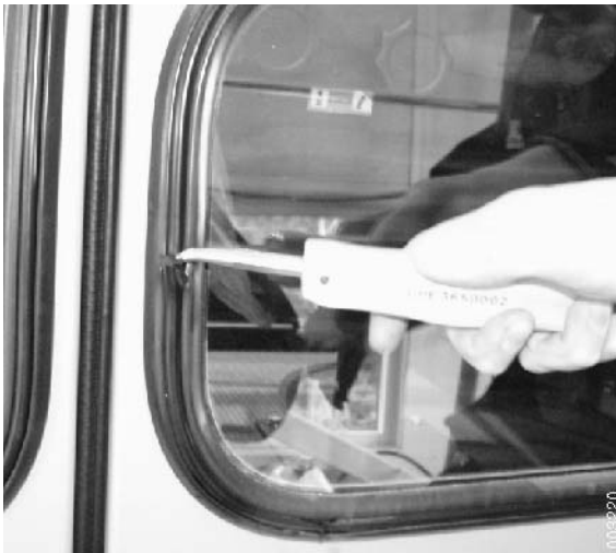
Figure 1: Removing key strip
