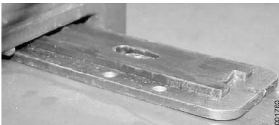
The illustration shows the inner slide plates in the attachment's main beam.
