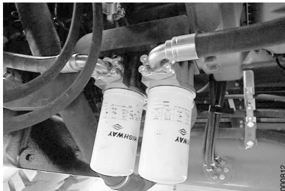
Oil filter transmission
