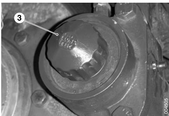
3. Casing parking brake
