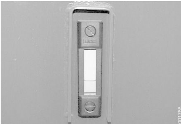
Relief valve for top lift, the figure shows an open valve.
