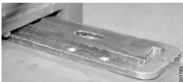
The illustration shows inner slide plates in the attachment's main beam.
