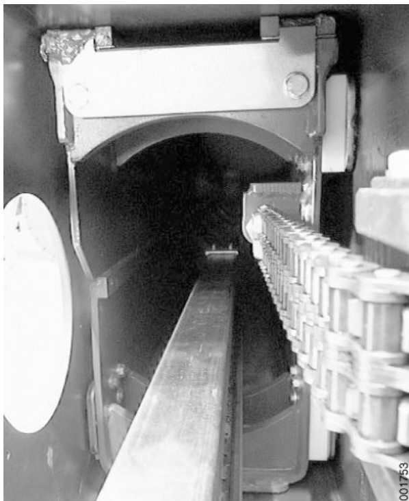
The illustration shows inner slide plates in the attachment's main beam.
