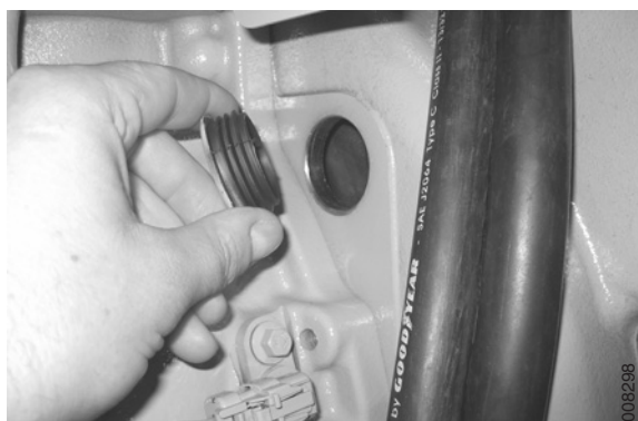
Bracket for the gearbox dipstick
