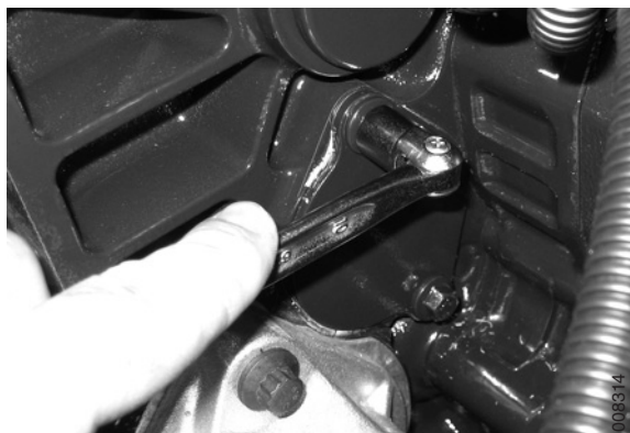
Bracket for the gearbox dipstick
