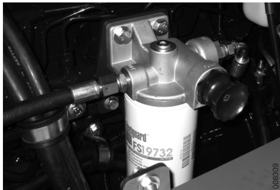
Fuel hoses on fuel filter
