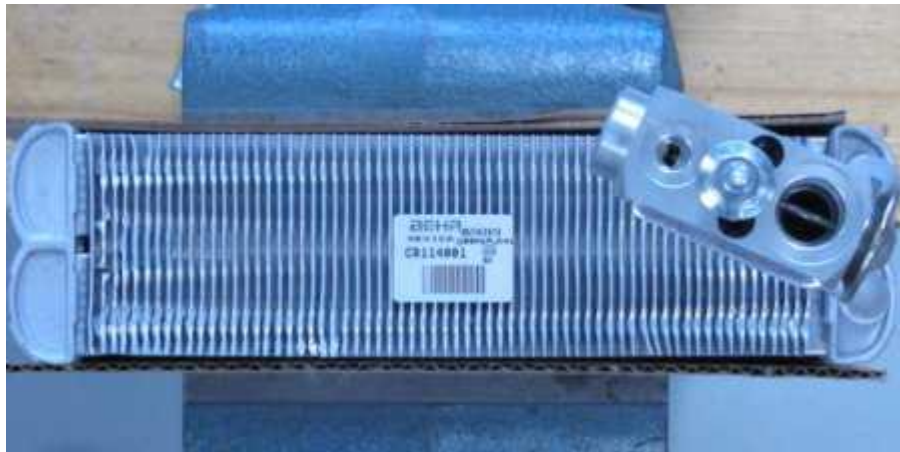
Finished Position of TXV Relative to Evaporator after Torque Applied
