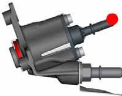
Figure 4-2: Measurement Location of DEF Dosing Module (Injector)
