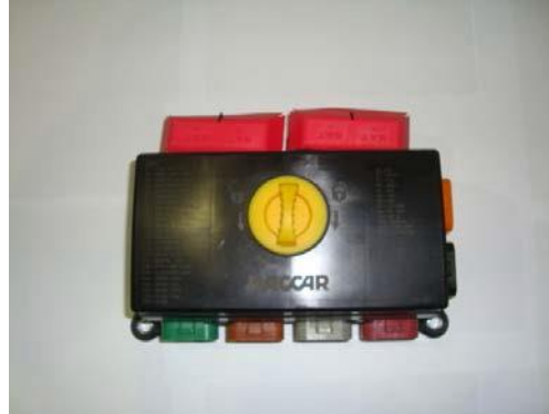
Figure 7.6.1 Power Distribution Center
