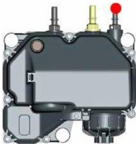
Figure 4-2 Measurement Location of DEF Supply Module (Pump)
