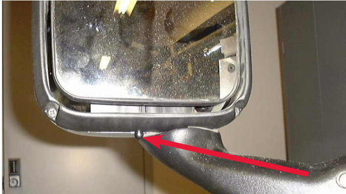
FIGURE 2-4: Aerodynamic Mirror OAT Sensor Location
