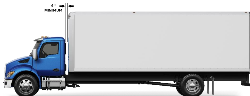
Figure 46 Minimum Back of Cab Clearance
