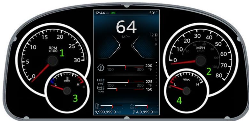
Figure 108 Gauges on the 7" Digital Display
