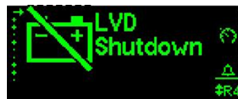
Low Voltage Disconnect
