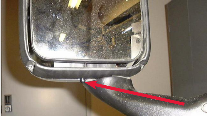
FIGURE 2-4: Aerodynamic Mirror OAT Sensor Location
