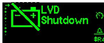
Low Voltage Disconnect
