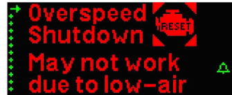
Engine Over-Speed Shutdown Low Air Warning
