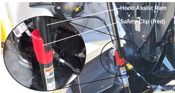
Hood Safety Latch shown in the safe position
