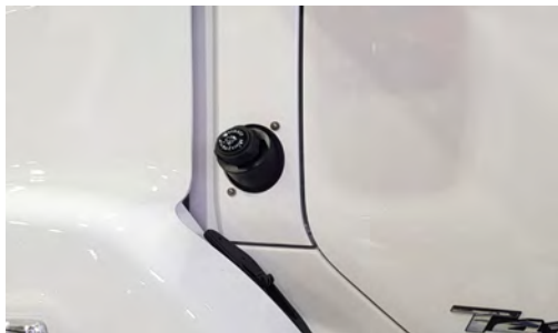
Windscreen Washer Reservoir Location on Left Hand Cowl Panel
