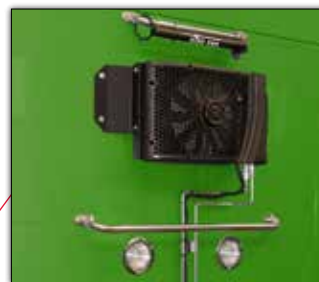
The remote condenser with brushless fan assembly is installed centrally on the upper exterior wall for optimum performance.
