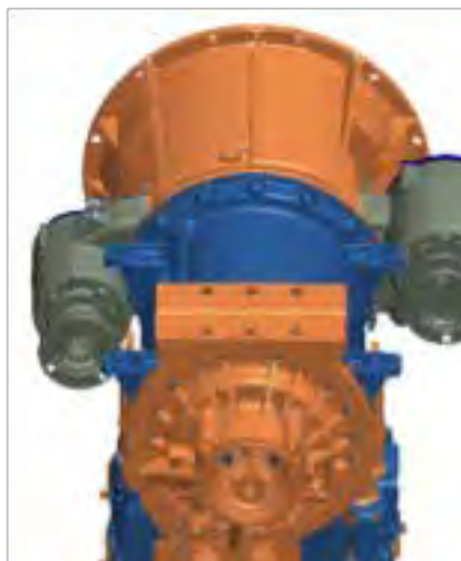
FIGURE 4-5. Allison 3000 Series Transmission PTO Locations
