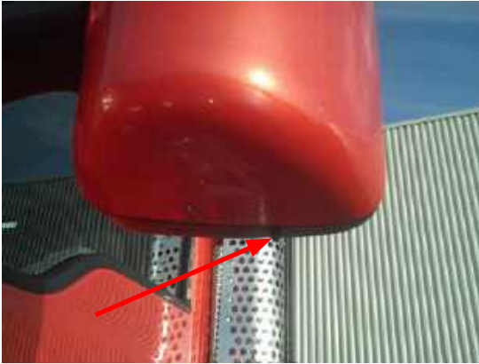
FIGURE 2-3: Aerodynamic Mirror OAT Sensor Location
