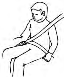
Incorrect (too high on hips)
