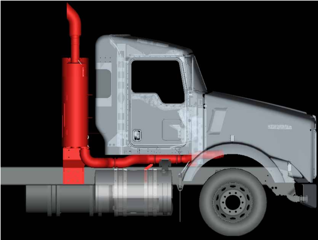
FIGURE 4-33: Right View of Vertical DPF and SCR
