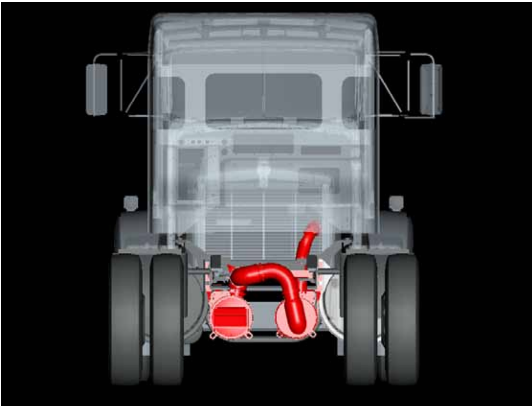
FIGURE 4-30: Back View of Horizontal DPF and SCR with Horizontal Tailpipe
