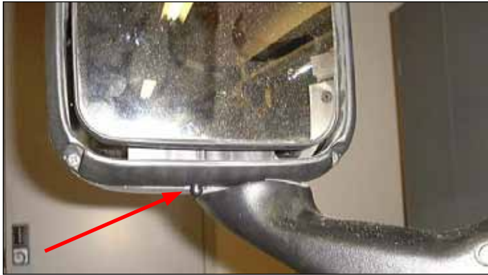
FIGURE 2-4: Aerodynamic Mirror OAT Sensor Location
