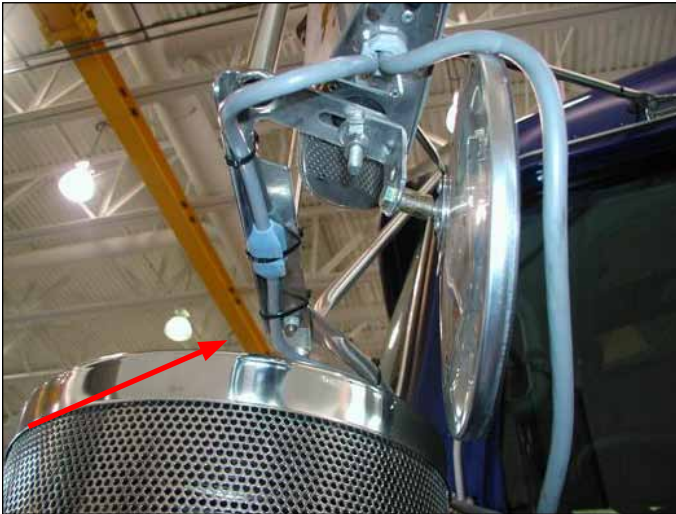
FIGURE 2-3: West Coast Mirror OAT sensor, located in overmold on mirror harness.
