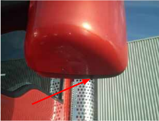
FIGURE 2-3: Aerodynamic Mirror OAT Sensor Location
