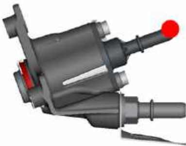
FIGURE 4-2: Measurement Location of DEF Dosing Module (Injector)
