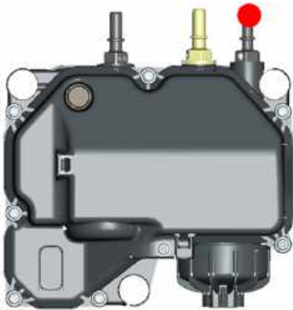
FIGURE 4-1: Measurement Location of DEF Supply Module (Pump)
