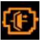
FIGURE 3-9. Rear Axle Declutch Telltale
