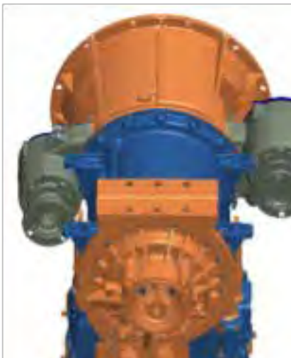
FIGURE 4-5. Allison 3000 Series Transmission PTO Locations
