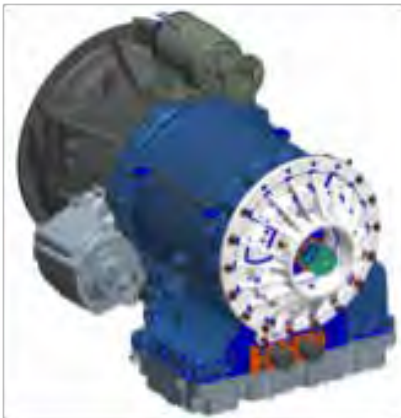
FIGURE 4-4. Allison 4000 Series Transmission PTO Locations
