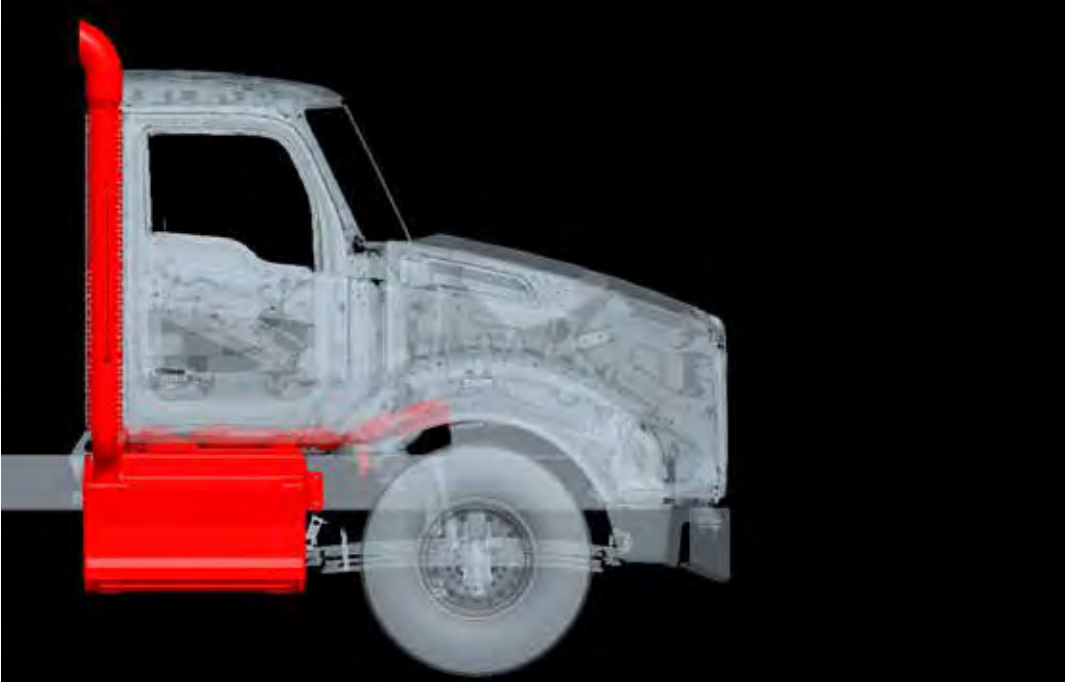
FIGURE 5-15: Right View of Right Hand Under DPF/SCR with Dual Side of Cab Tailpipe
