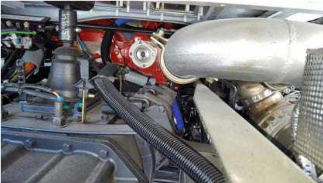
FIGURE 4-4. REPTO Flywheel Housing
