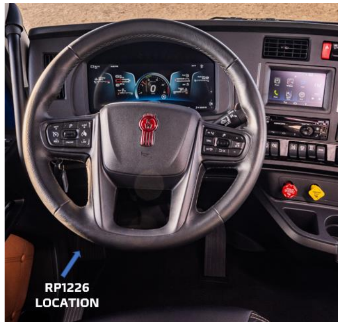
FIGURE 10-4. RP1226 Location (Driver's Side Kick Panel)
