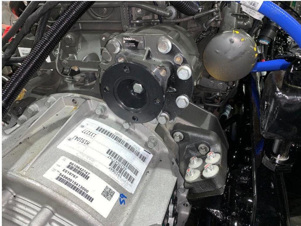
Figure 4-3. REPTO Flywheel Housing
