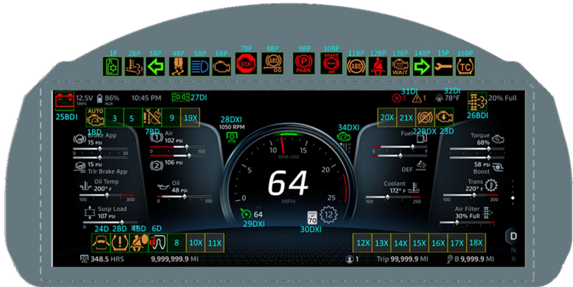
Figure 2-4 Digital Dash (15in) for T680/T880/W990 (EPA 2021+)
