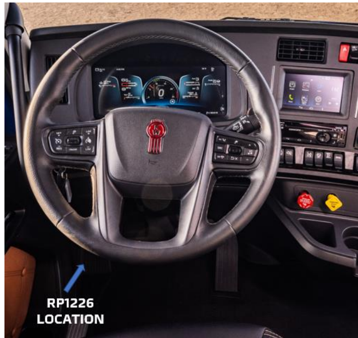
Figure 4-15. Standard RP1226 Location (Driver's Side Kick Panel)
