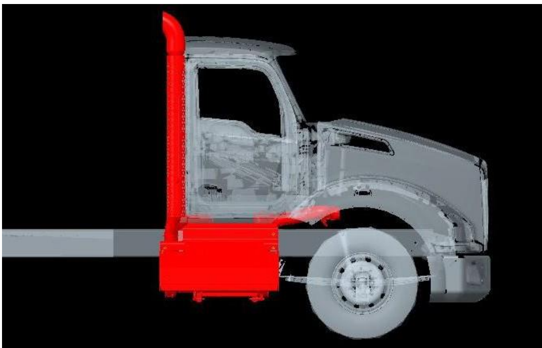
FIGURE 5-12. RHUC DPF/SCR Dual SOC Tailpipes – RH View
