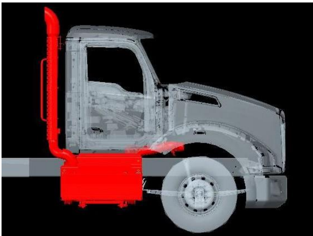
FIGURE 5-16. RHUC DPF/SCR BOC Tailpipe – RH View
