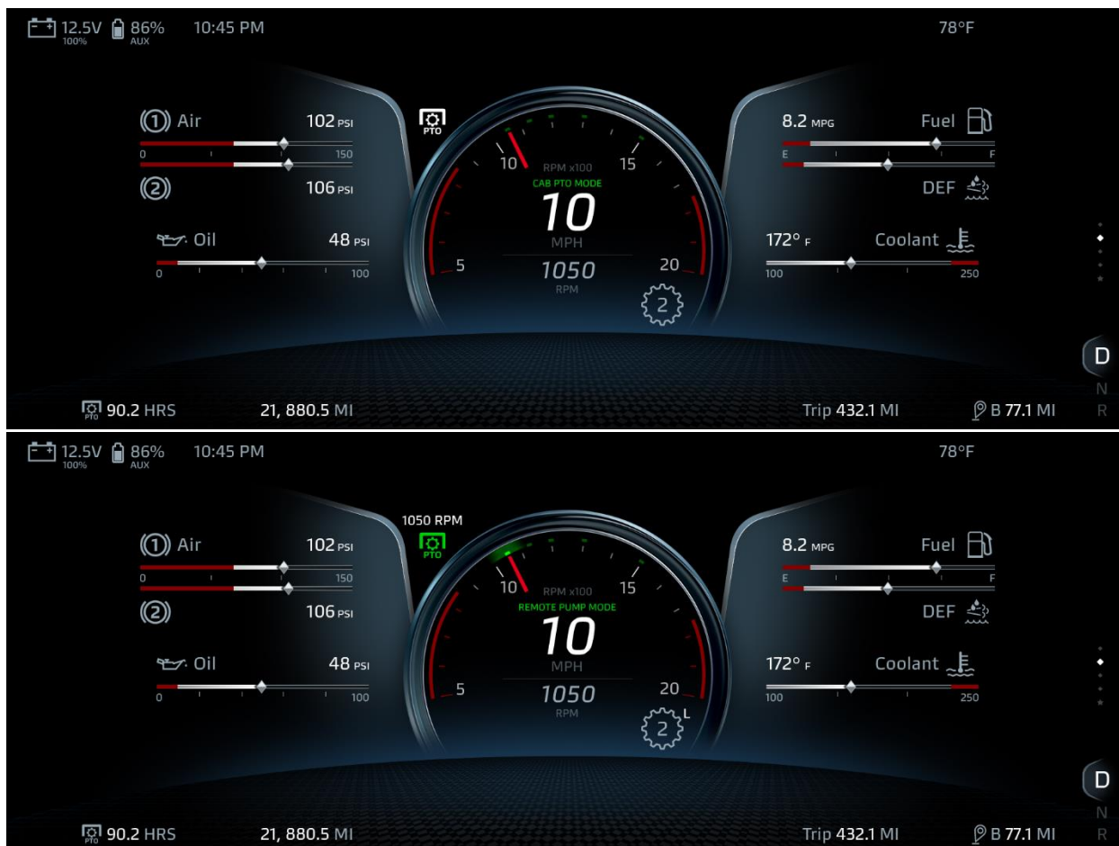
Figure 4-5. PTO Telltale Location (15in Digital Display)
