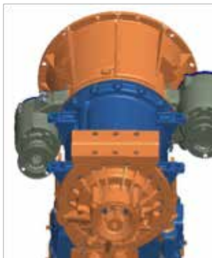
FIGURE 4-5. Allison 3000 Series Transmission PTO Locations
