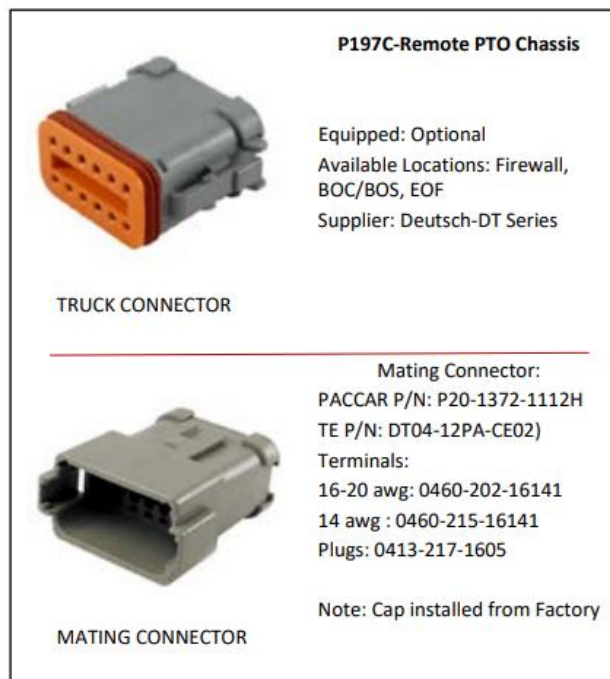
FIGURE 10-14. P197C (12-Pin) Connector and Mating Connector Information
