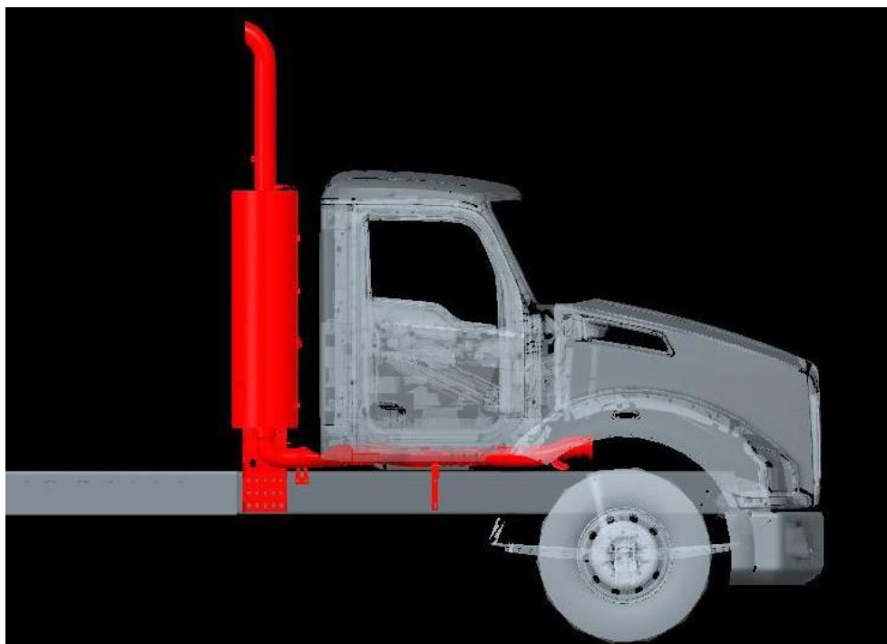
FIGURE 5-24. Independent BOC DPF/SCR w/BOC Tailpipe – RH View
