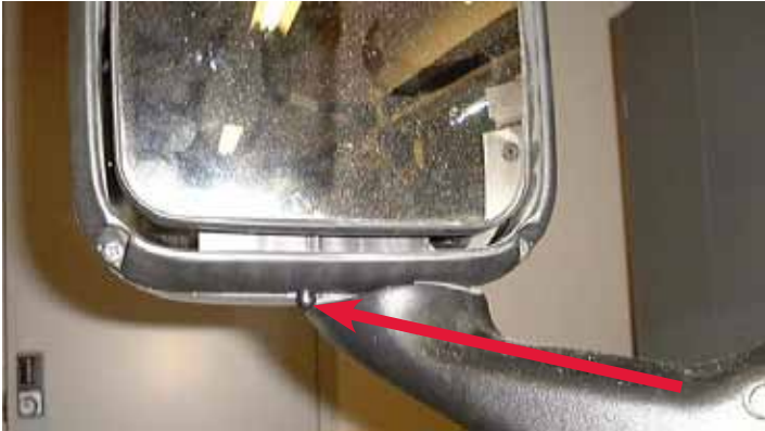
FIGURE 2-4: Aerodynamic Mirror OAT Sensor Location
