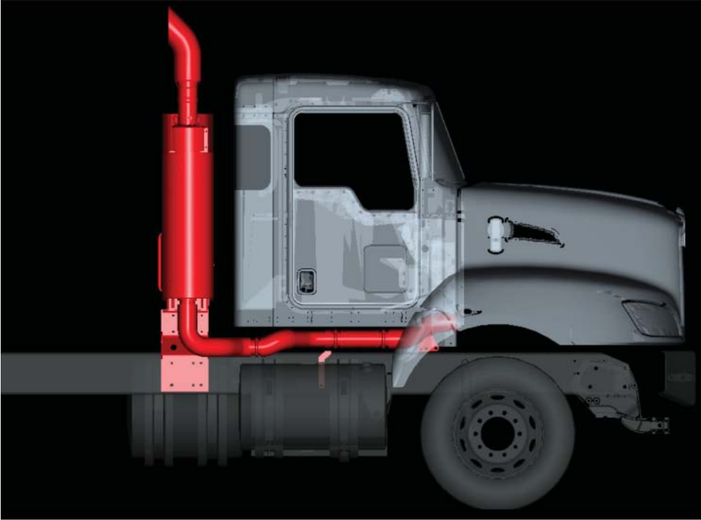
FIGURE 4-20: Right View of Vertical DPF and SCR
