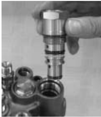
Install the holder with new O-ring, (timer).
