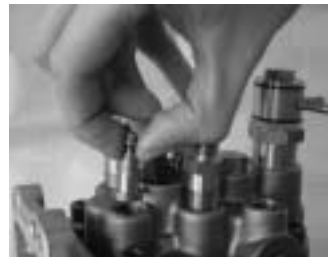
Remove the delivery valve and gasket.
