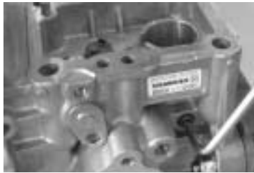
Remove the whirl-stop, (tappet).
