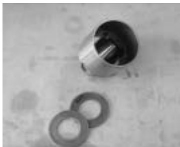
Tappet disassembled and FIC adjust shim.
