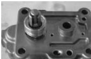
Install the control sleeve and spring retainer.
