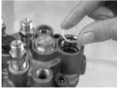
Install the new packing, (timer).
