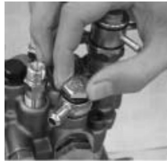
Install the joint, (FO inlet).
