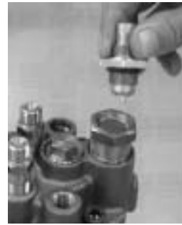
Install the thermo-element with new O-ring.
