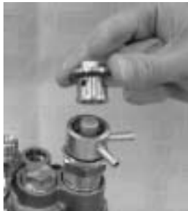
Install the joint, (C.W.), and the plug, (C.W.)
