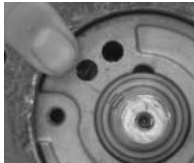
Align the camshaft's key groove with the embossed mark on the body.
