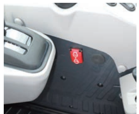
Secondary engine shutdown switch
