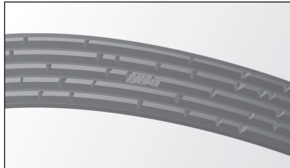
Belt With Severe Cracking
