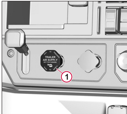
1 Trailer Air Supply
