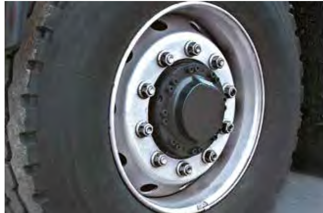
Front axle with hydrostatic wheel hub motors
