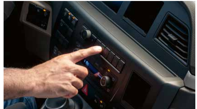
Freely programmable direct access buttons fitted with touch sensors
