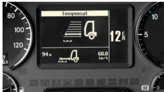
The Telligent® proximity control optionally available in conjunction with a retarder allows more relaxed and safe driving. This is because the speed and gap maintained by the Actros are automatically adjusted by the drive and braking cruise control as the traffic situation changes.
