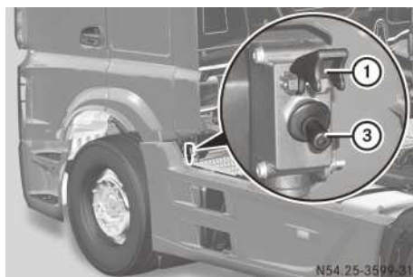
Example: battery isolator switch
