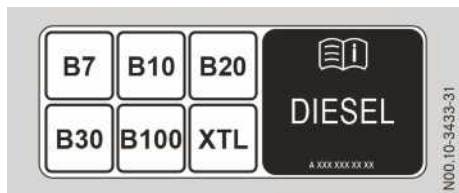
Compatibility labels only for BlueTec® vehicles with OM471 engines (code MOW)
