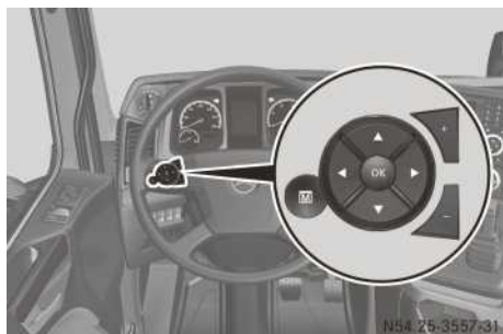
Left group of buttons on the multifunction steering wheel
