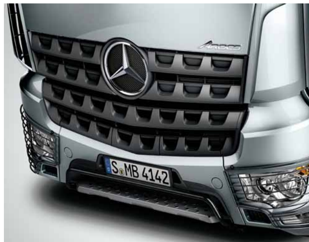
Radiator grille with excavator tooth design
