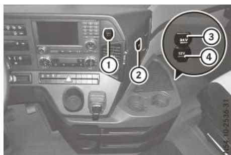
Example: power sockets on the dashboard
