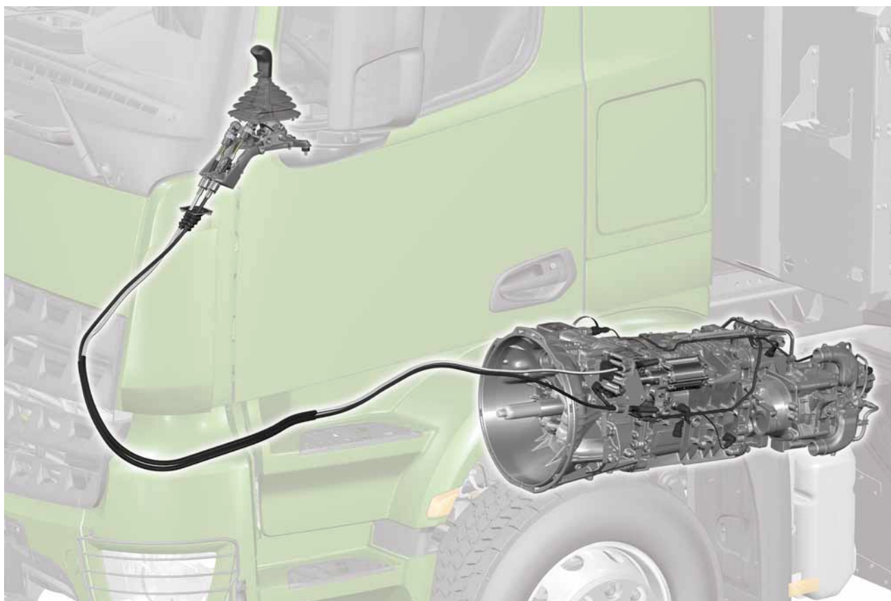
Overview of cable shift (illustrated on the 6x4 dumper)
