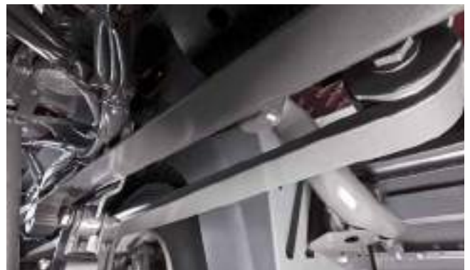
Rear spring, 5.0 t, parabolic, 1-leaf (Q2N)
