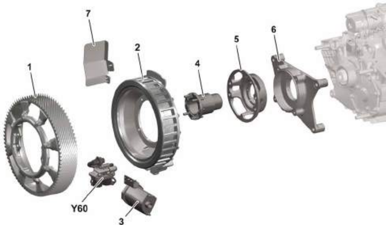
Permanent magnet retarder (B3G) on transmission G 90-6
