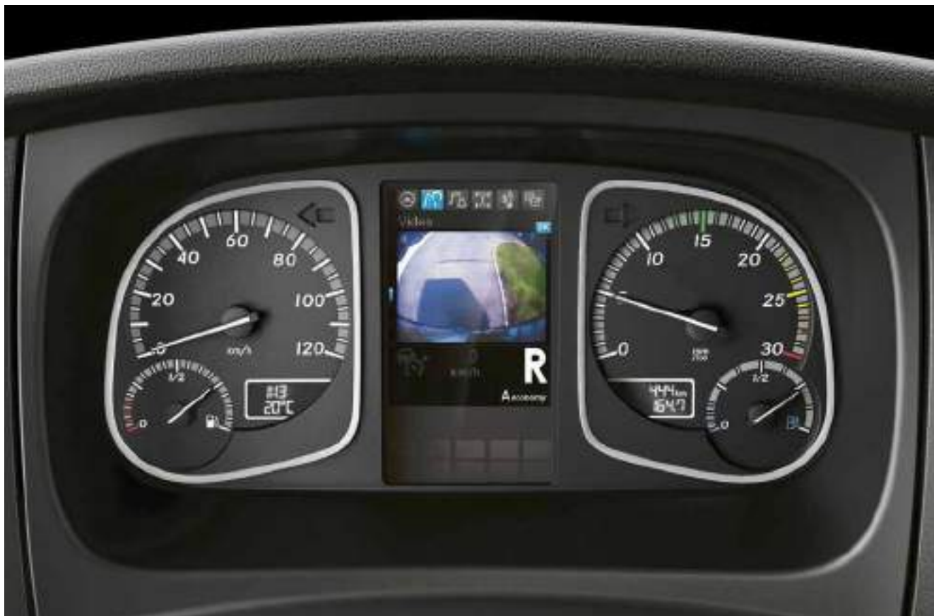
Instrument cluster 12.7 cm, with video function (J1C)
