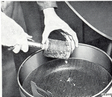
Fig. 27 Cleaning of fuel filter element
