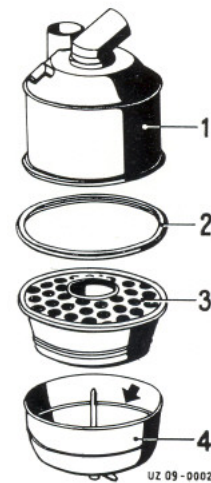
Fig. 20 Oil bath air filter, disassembled
