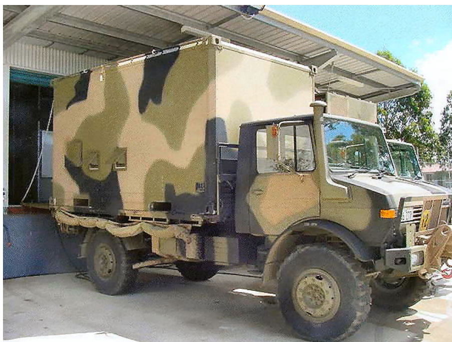
Figure 9D-3: Unimog Maintenance Shelter
