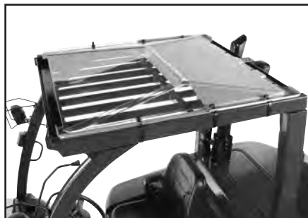
Polycarbonate rain guard, with water diversion channels, partially opaque for protection from the sun.
