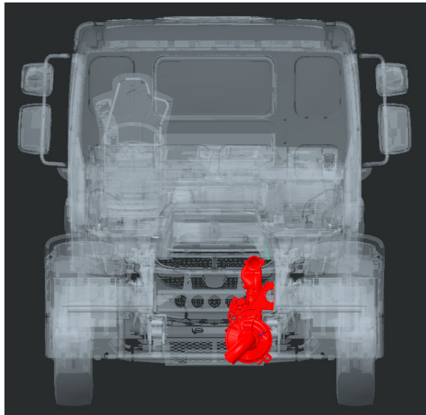
Figure 4-6.4 Back view of Horizontal Exhaust Canister with Horizontal Tailpipe
