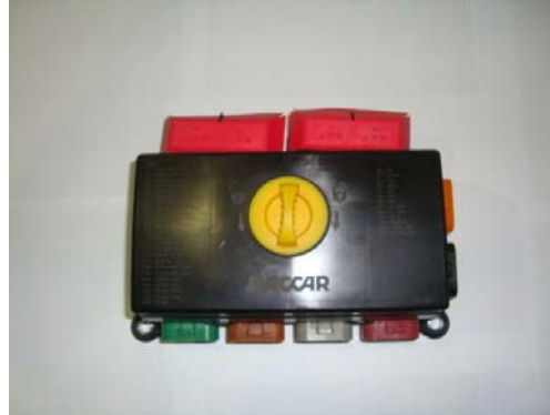
Figure 7.6.1 Pwer Distribution Center
