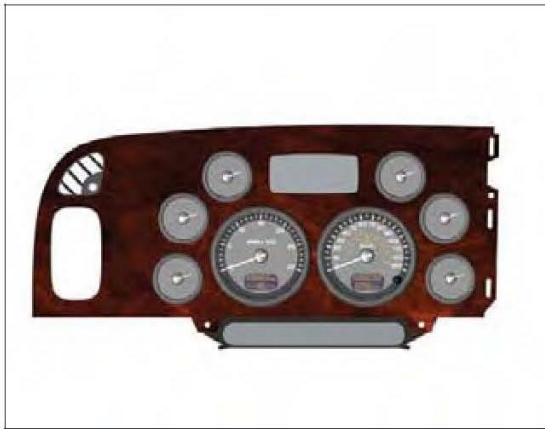
"A" Panel with Cluster Installed Removed
