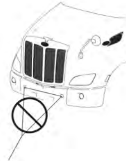
3. NEVER USE SINGLE CHAIN OR CABLE LOOPED THROUGH TOW DEVICES
