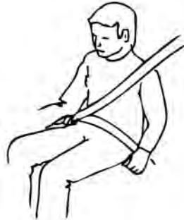
Incorrect (too high on hips)
