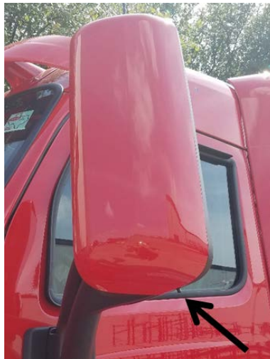
FIGURE 2-3: Aerodynamic Mirror OAT Sensor Location
