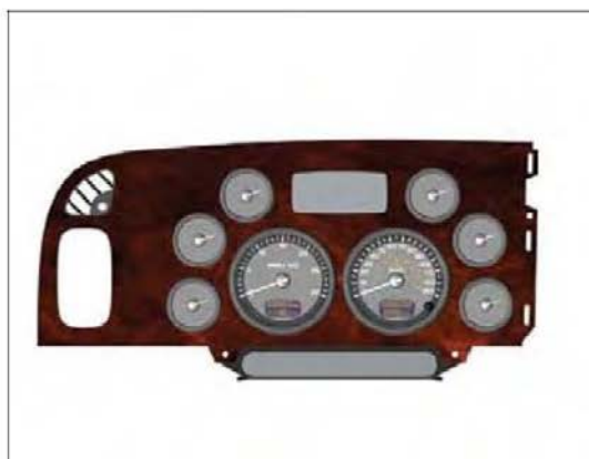
"A" Panel with Cluster Installed
