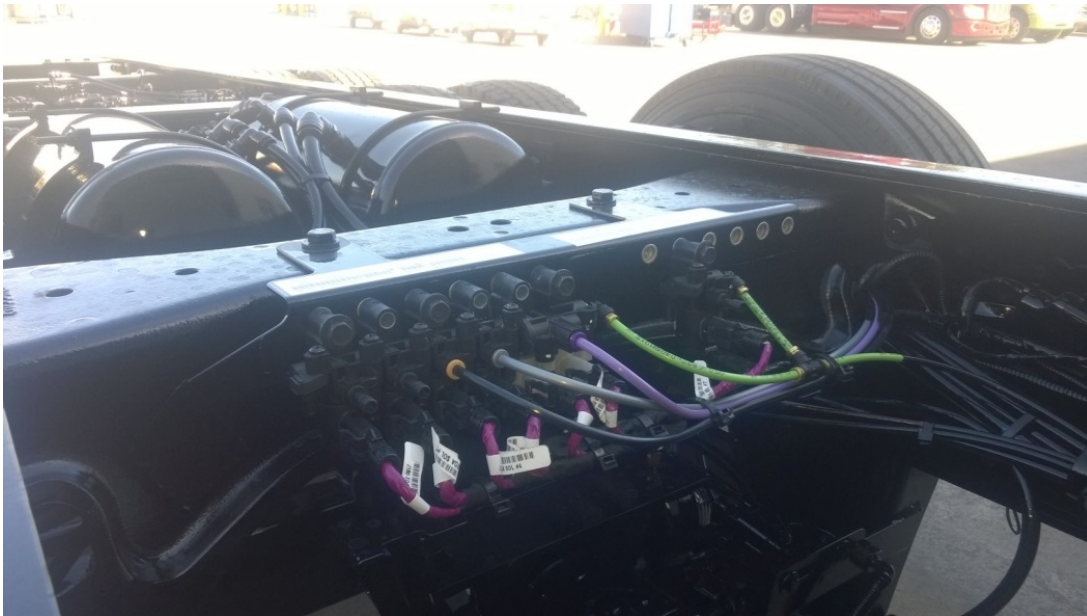
FIGURE 7-45. EOA Solenoid Location for Chassis Built After 1/1/2016
