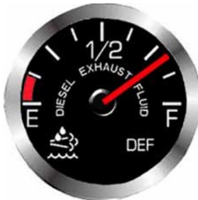
FIGURE 6-3. Diesel Exhaust Fluid Gauge
