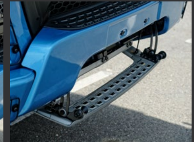
Folding anti-slip platform for better windscreen accessibility.
