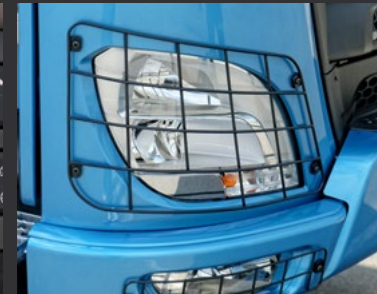
Protective grilles for LED headlamps and fog lamps.
