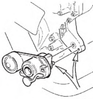
Fig. 127: Install the belt tensioner
