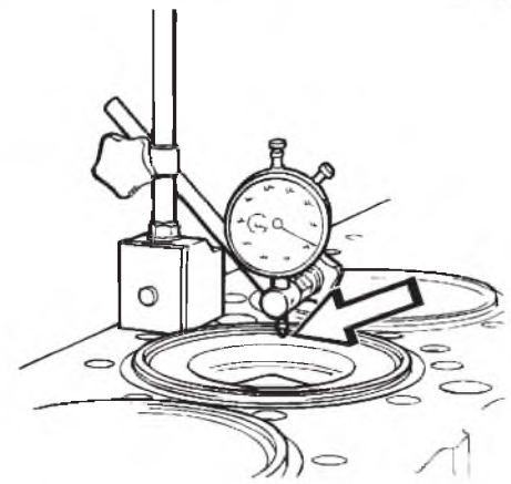
Fig. 10: Measuring the height of the piston
