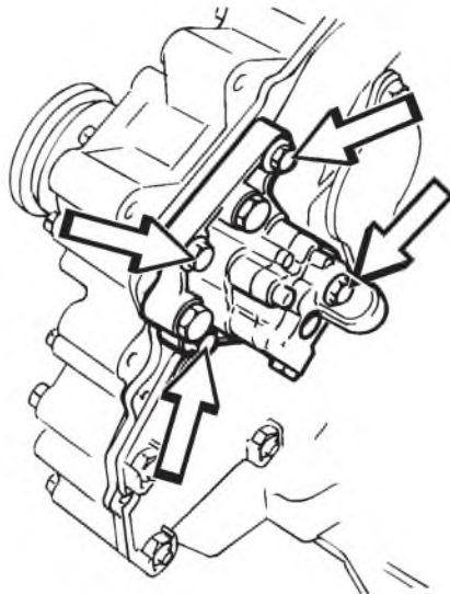
Fig. 46: Removing fuel pump
