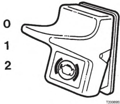
Fig. 10: Switch for engine brake
