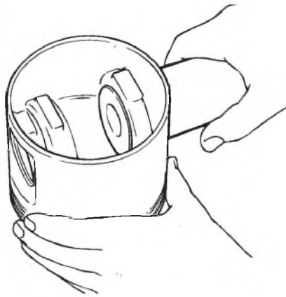
Fig. 5: Installing the piston pin
