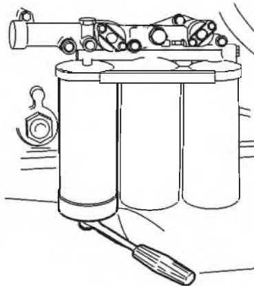
Fig. 17: Replacing oil filters
