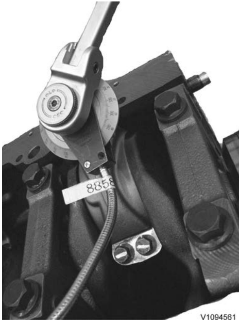
Fig.63 Tightening down bearing cap
